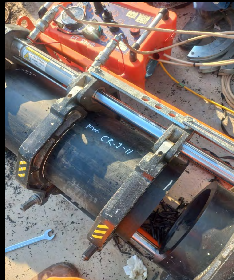
BUTT FUSION PROCESS
