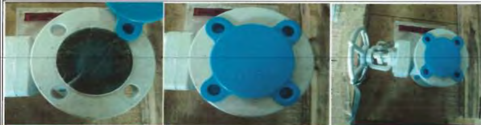
Preservation Cleaning, Greasing & Covering For Manual Valve
